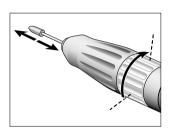
Turn the expansion ring clockwise up to the limit stop. Push in the rotary tool up to the limit stop or remove.
