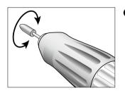
Start the motor handpiece until the required speed is reached. After approx. 2 seconds, an audible signal sounds and the required speed is saved.
