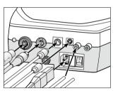
Connect the motor cable, operating controls, foot-operated starter, air hose, coolant hose (control unit with external coolant supplying) and mains cable.
