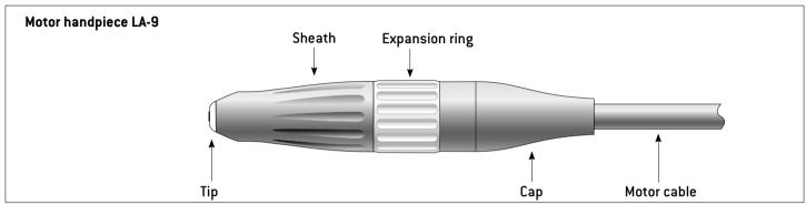
The milling device adaptor (optional) for the motor handpiece can be fastened above or below the expansion ring.
