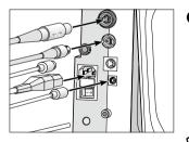
2 Connect the motor cable, operating controls, air hose, foot-operated starter (optional), coolant hose (control unit with external coolant supplying) and mains cable.
