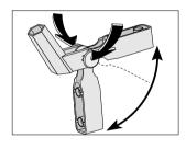
The support (optional) can be moved into a variety of assembly positions by simultaneously pressing both buttons on the joint.
