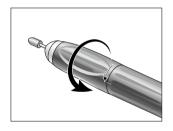
Turn the front sheath anticlockwise until it engages audibly.
