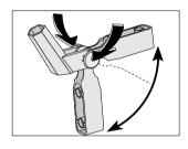
The support (optional) can be moved into a variety of assembly positions by simultaneously pressing both buttons on the joint.
