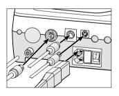
Ocnnect the motor cable, operating controls, footoperated starter, air hose (Perfecta 600) and mains cable.
