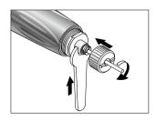
1 Insert the chuck key up to the limit stop in the chuck and screw clockwise.
