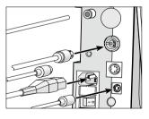
Connect the motor cable, operating controls, footoperated starter (optional), air hose (Perfecta 600) and mains cable.
