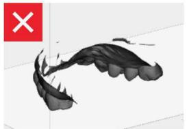
Non-Printable Data Direct scanned data will be displayed as open mesh in SprintRay Software. This data requires 3rd party software to make it printable.
