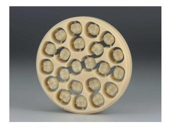
For milling with the aid of open CAM systems, SHOFU Disk HC circular blocks, 98.5 mm in diameter, are also available.
