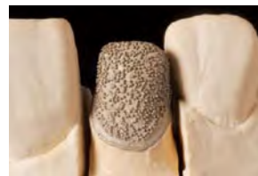
Metal framework after sandblasting with aluminium oxide
