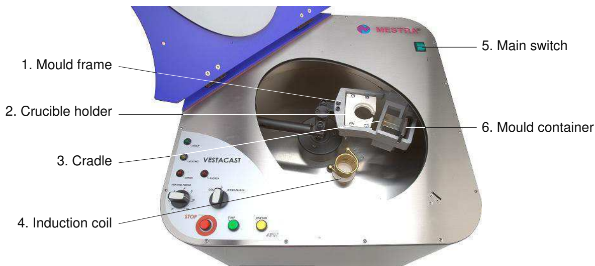
Fig. 2: Casting chamber with centrifugal arm
