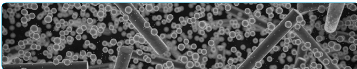
Figure 2: everX Flow is based on fibres and particle fillers in a resin matrix (computer-generated image)
