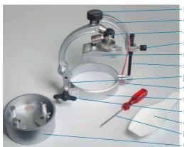
press button occludating bow arresting joint supporting pin fixation model plate supporting pin joint column fixation screw fixation ring swing bolt granules shovel hex-wrench size 3 model pot
