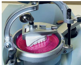
9. Close the Occluform-3 to the stop, wait for the cooling time.
